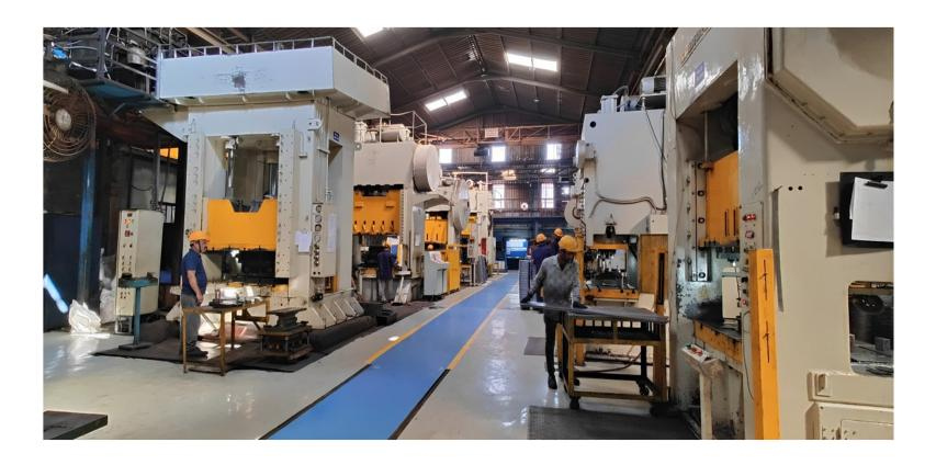
Equipped with mechanical and hydraulic presses (160 to 500 tons) for tool try-outs and solutions for regular and batch production
